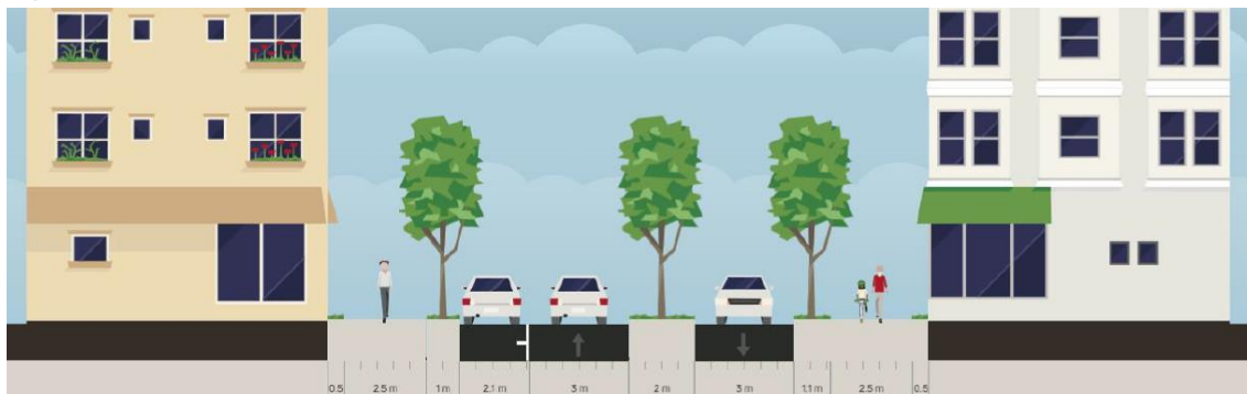
Figure 4.3: 18.2m Main Street Cross Section
