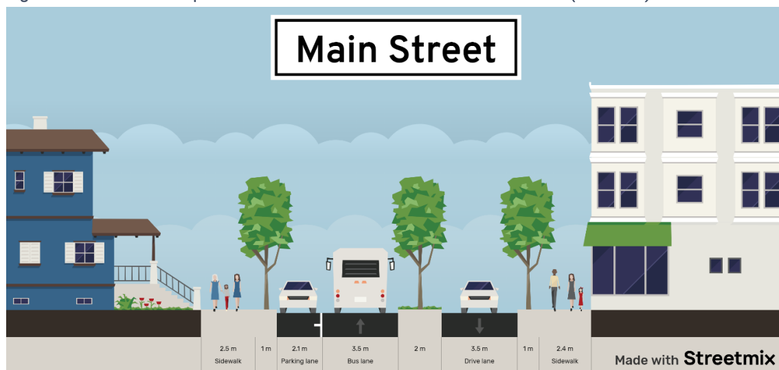
Figure 4.5: Indicative Representation of an 18m Main Street Cross Section ( Streetmix )
