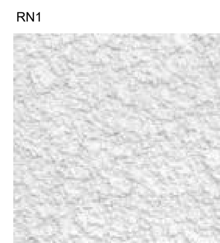
RN1 OFF WHITE TEXTURED RENDER; UNITEX SPRAY COARSE (DASH) COAT OR SIMILAR
