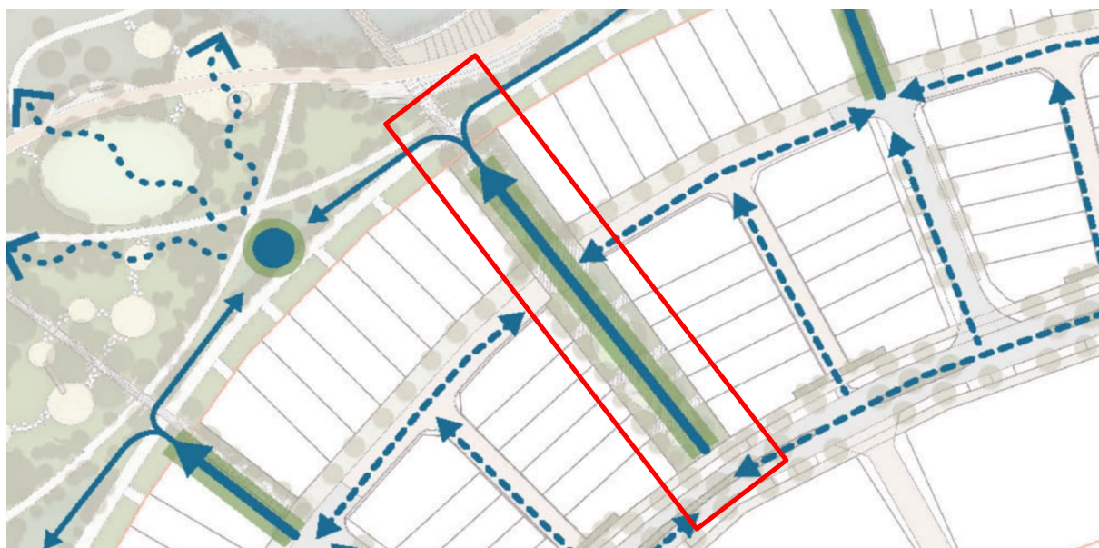
Figure 7 - Stormwater Drainage Concept Plan – Showing drainage flow paths (piped & swales ) and disposal routes incorporating biofiltration and & Storage.
