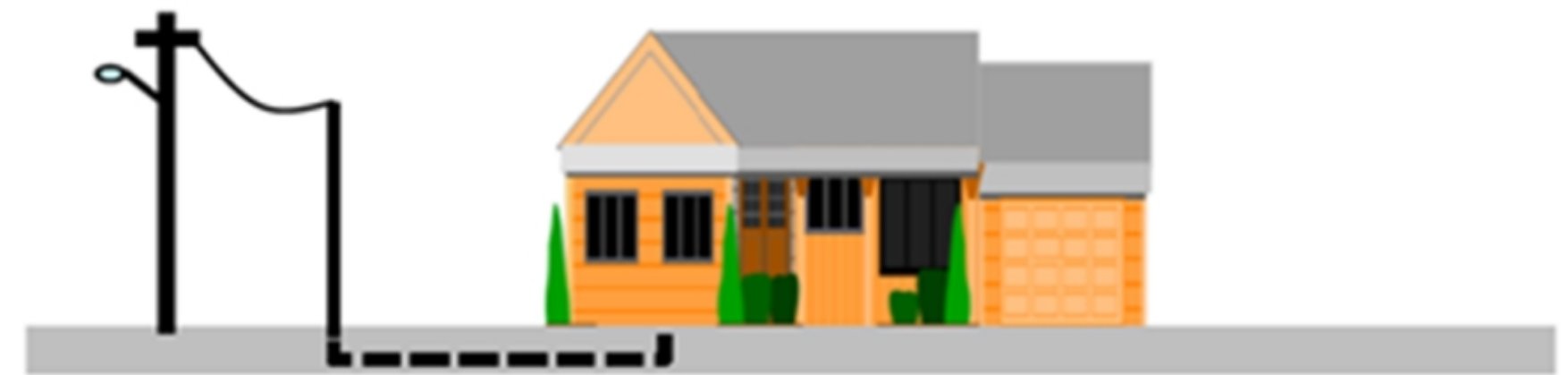
UNDERGROUND FROM SERVICE POLE
