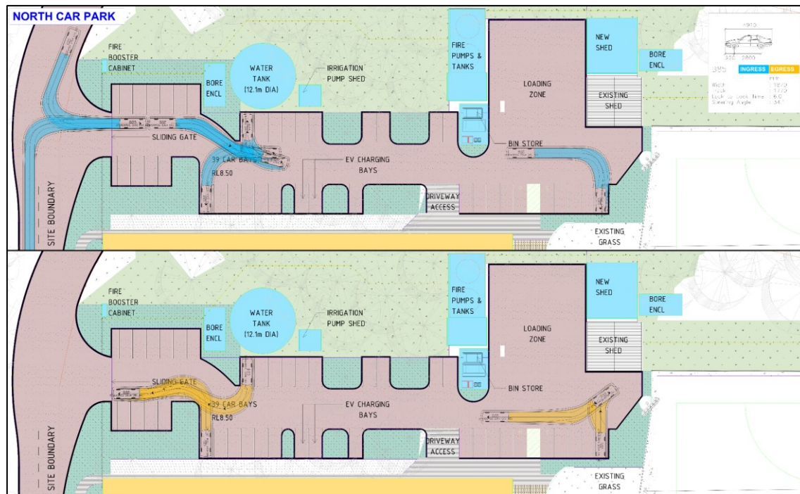
Figure 5-3: Swept Paths – B85 Design Vehicle (North Car Park)
