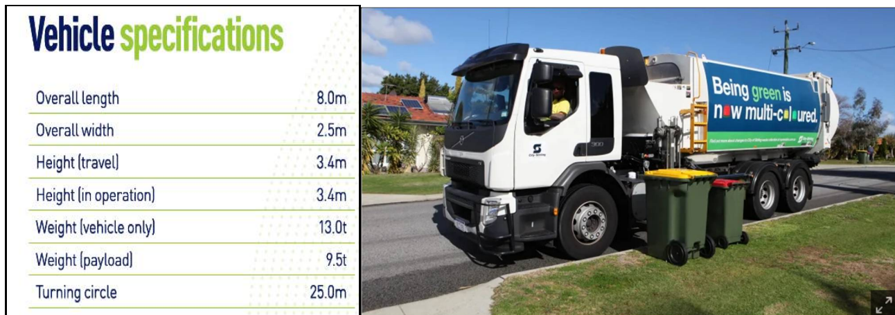
Figure 2 – Rubbish truck & approximate specifications to be adopted for the development (verge pick up).
