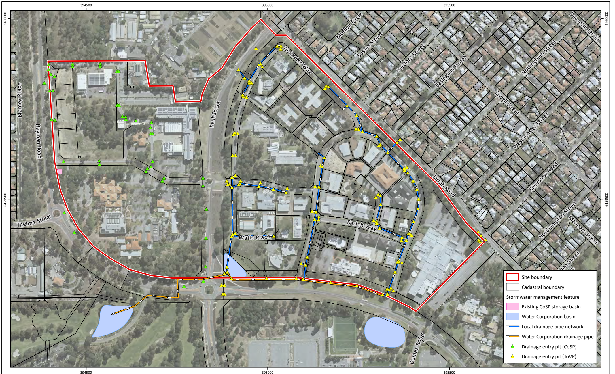
Figure 4: Existing Hydrology and Local Drainage Network
