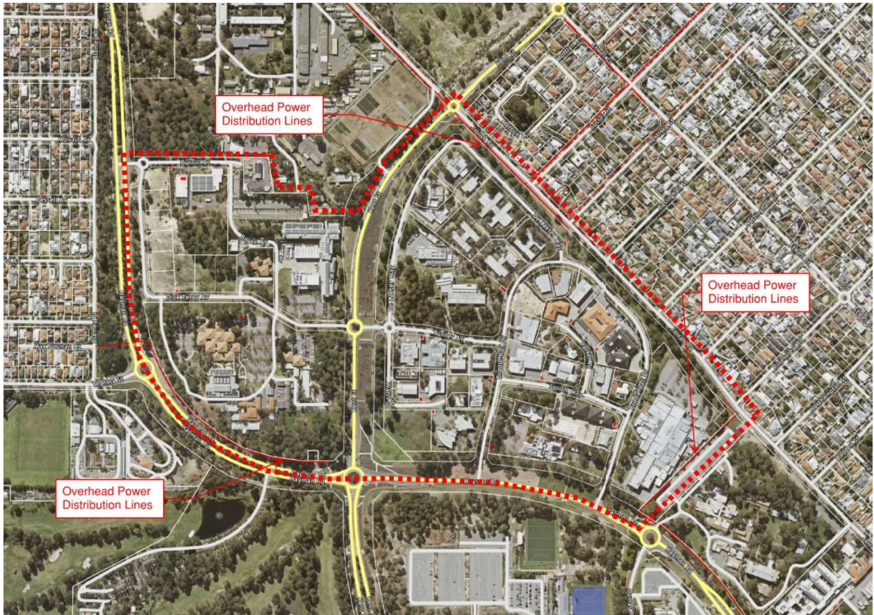
Figure 7 – Western Power Overhead Power Distribution. September 2025 (MNG Access)
