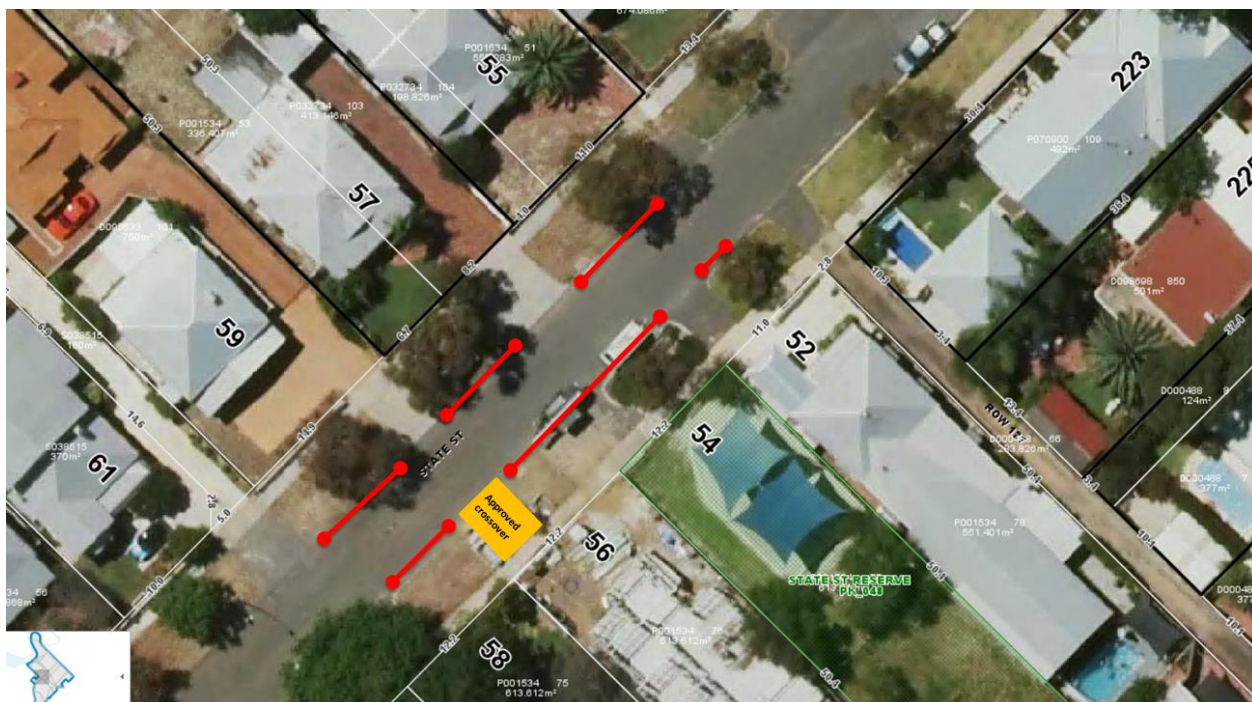
Figure 2 Indicative on-street parking restrictions for accommodating a pedestrian median island
