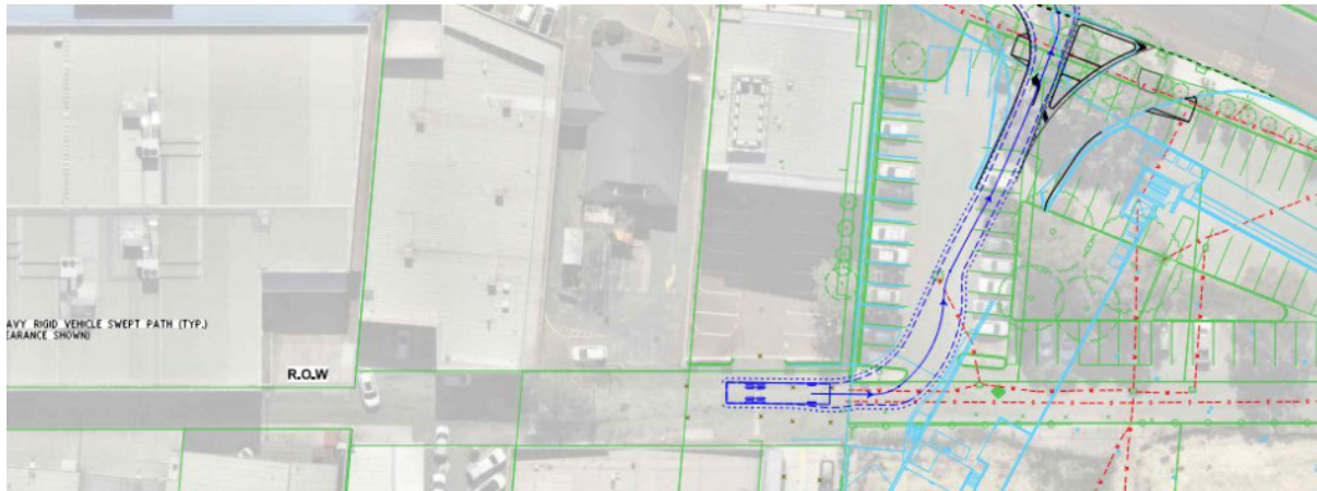
Figure 2 – Extract from TIS showing 12.5m HRV travelling east along ROW54
