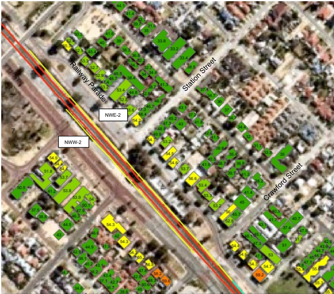
FIGURE 7 NOISE WALL LOCATION REQUIREMENTS FOR LXR PROJECT
