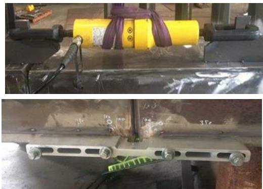
Figure 26: Typical Hydraulic Pull Cylinder and Bolting Frame
