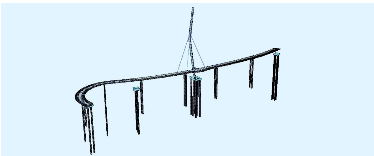
Figure 13 Construction Stage Model - Cable C26 Installation Stage
