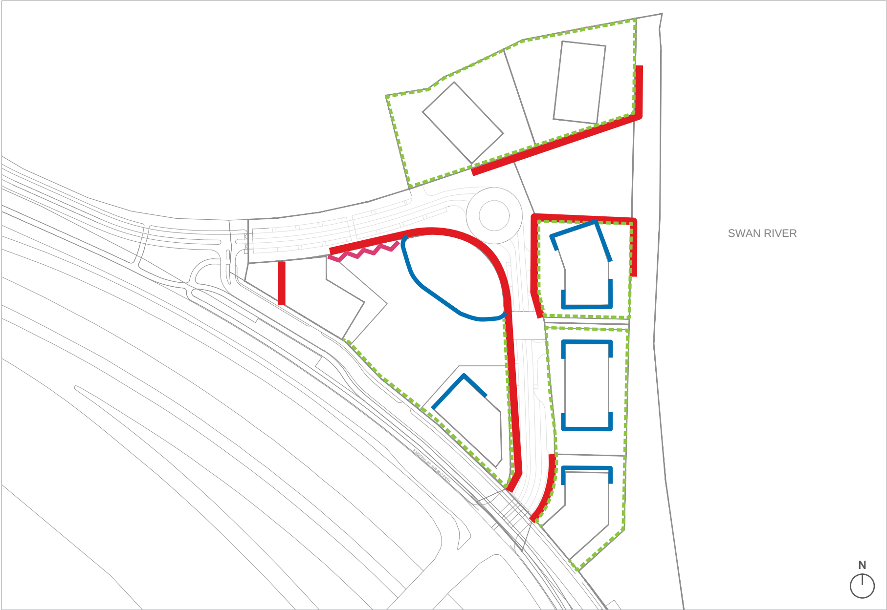
Figure 62: Design elements required to minimise wind impacts. The awnings identified in this drawing are required to mitigate wind impacts. Awnings are also required in other areas, as stipulated in the Site Specific Guidelines. Note: These design solutions are provided as guidance and alternative approaches may be approved where they are supported by a wind impact statement.
