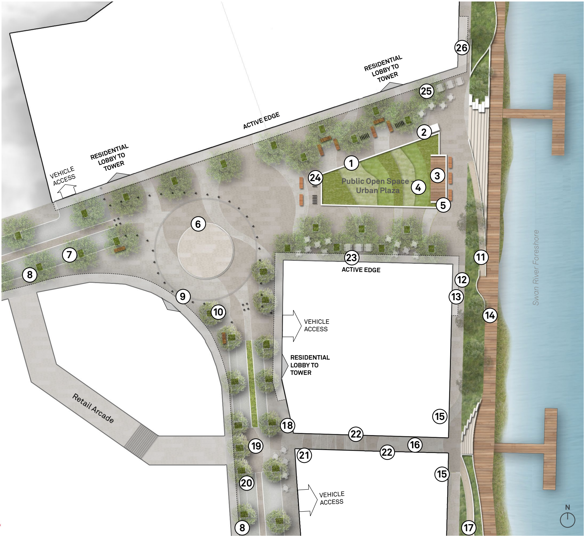
Figure 88: Detailed Plan of the urban plaza describing its intended function. Detailed design during subdivision stage will determine exact characteristics and design detail. Note: drawing is notional to help describe general requirements and intended function.
