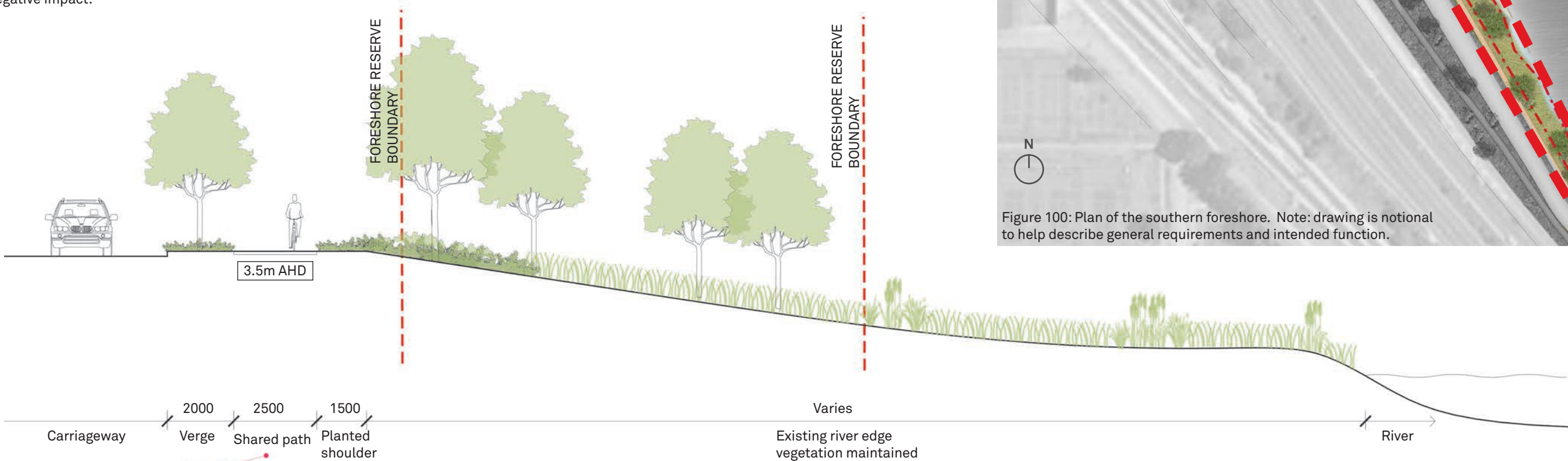
Figure 101: Section drawing of the southern foreshore in the area indicated. Note: drawing is notional to help describe general requirements and intended function.
